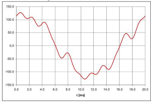
A harmonic load has the following current waveform:
