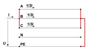
Phase - PE (earth wire) measurement
