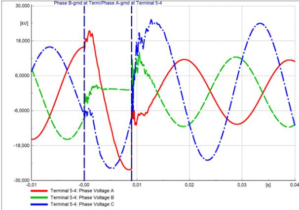
Figure 17: Phase voltages at Terminal 5-4.
