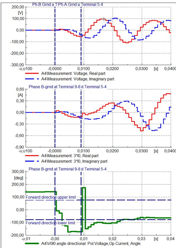
Figure 18: A4 relay,  $U0x3$ ,  $I0x3$  and  $U0V0$  angle signals.
