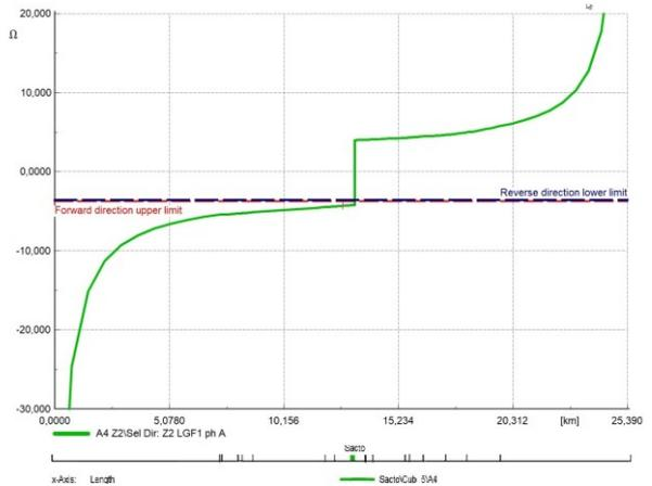
Figure 13:  $Z_2$  at A4 measured for a single phase-ground fault moving along the MV loop (phase A)
