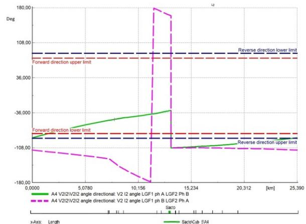
Figure 10:  $12V_2$  angle at A4, CCF with  $LGF_1$  at Sacto,  $R_f=15 \Omega$
