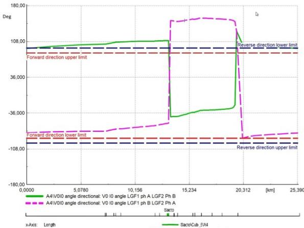
Figure 8:  $10V_0$  angle at A4, CCF with  $LGF_1$  at Laganà,  $R_f=15 \Omega$
