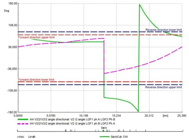
Figure 9:  $12V_2$  angle at A4, CCF with  $LGF_1$  at Terminal17-16 between Taurianova and Sacto,  $R_f=15 \Omega$
