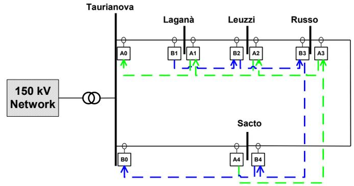
Figure 3. Protection system with permissive overreach blocking logic.
