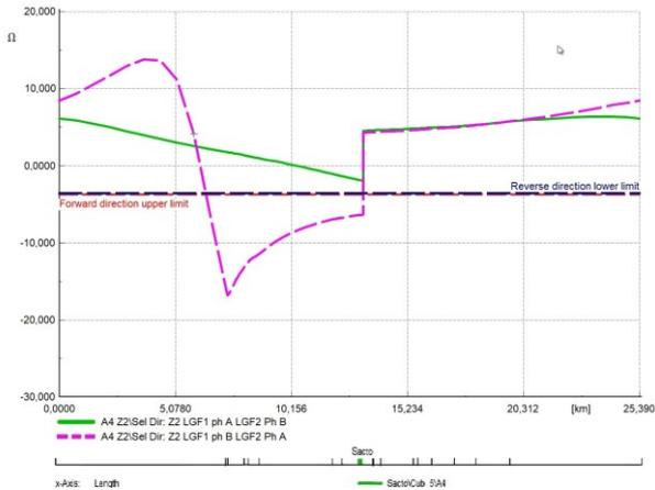
Figure 16: Z<sub>2</sub>, CCF with LGF<sub>1</sub> at Laganà busbar, R<sub>f</sub>=15 Ω, LGF<sub>2</sub> moving along the MV loop R<sub>f</sub>=15 Ω
