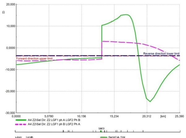
Figure 14:  $Z_2$  CCF with  $LGF_1$  at Terminal 17-16,  $R_f=15 \Omega$ ,  $LGF_2$  moving along the MV loop,  $R_f=15 \Omega$
