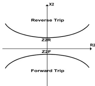
Figure 12:  $Z_2$  directional characteristic
