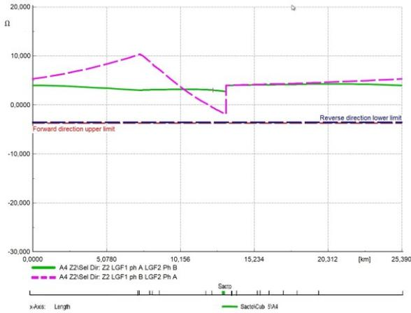
Figure 15: Z<sub>2</sub>, CCF with LGF<sub>1</sub> at Sacto busbar, R<sub>f</sub>=15 Ω, LGF<sub>2</sub> moving along the MV loop, R<sub>f</sub>=15 Ω
