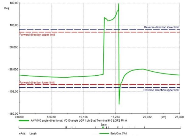
Figure 5:  $10V0$  angle at A4, CCF with LGF<sub>1</sub> at Load 5-6, Phase B,  $R_f=15 \Omega$
