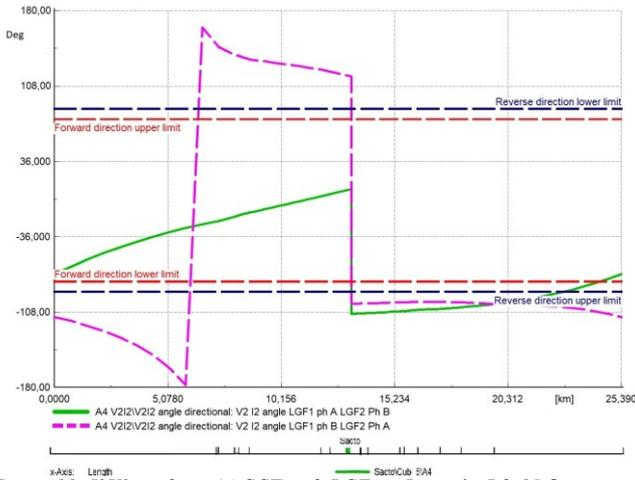
Figure 11:  $I2V2$  angle at A4 CCF with  $LGF_1$  at Laganà,  $R_f=15 \Omega$
