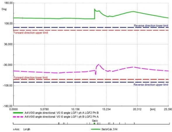
Figure 7:  $10V_0$  angle at A4, CCF with  $LGF_1$  at Sacto,  $R_f=15 \Omega$
