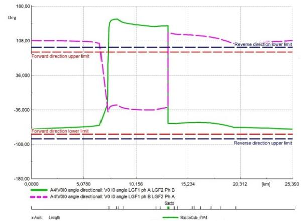
Figure 6:  $10V0$  angle at A4, CCF with LGF<sub>1</sub> at Terminal 17-16 between Taurianova and Sacto,  $R_f=15 \Omega$
