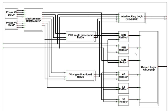
Figure 4. RGDM relay model connection scheme
