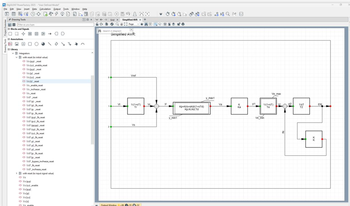
Figure 6: Example of a DSL model using block diagrams
