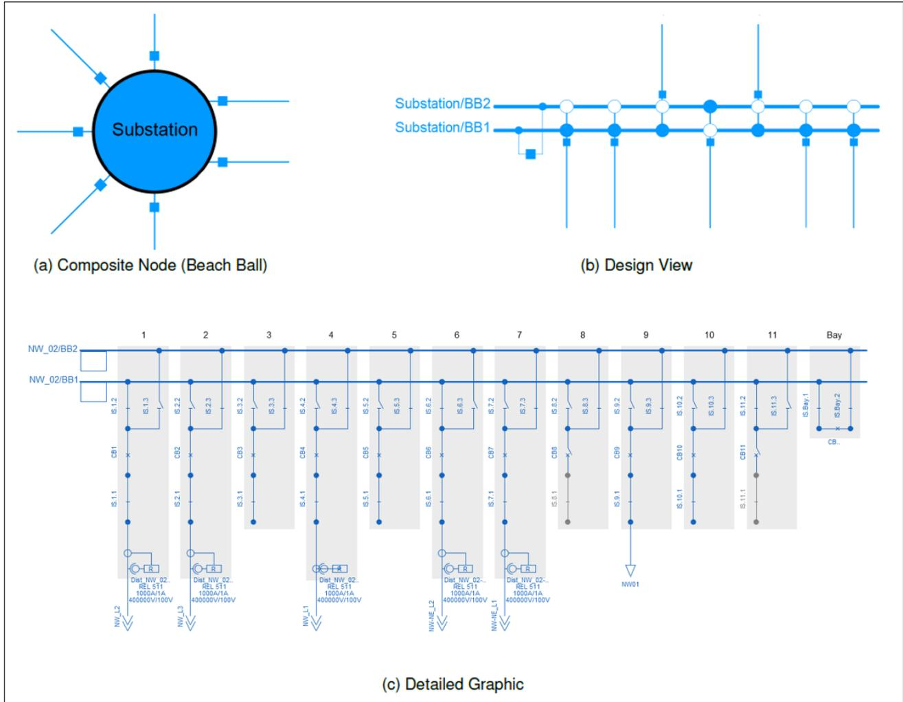
Figure 4: Substation graphical representations
