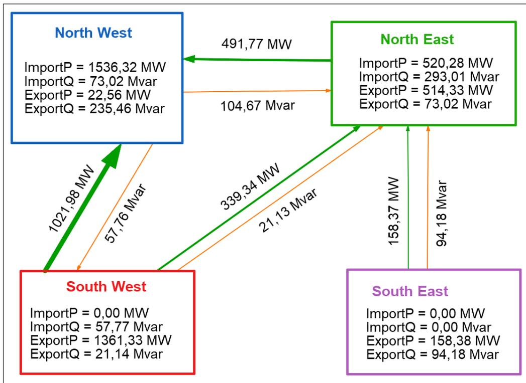
Figure 3: Area interchange diagram
