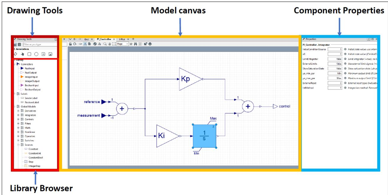
Figure 7: Overview of the Modelica models graphical environment
