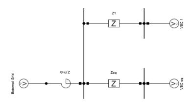
Figure 1: Basic equivalent circuit applied for model aggregation of a power park containing "n" units arranged in a radial topology.
