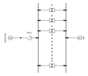
Based on the above circuit, an equivalent impedance can be calculated  $Z_{\it eq}$ :
