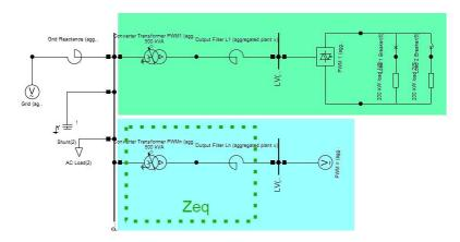
Nevertheless, it is important that the equivalent impedance is adequately modelled. The simplest method to do that is to duplicate the output filter of the VSC, along with the transformer and optionally any output cable stepouts and make use of the number of parallel units parameters of these built-in components. Note, some elements do not have a parameter for parallelisation e.g. ElmSind. In such cases, manual computation of the equivalent impedance is required.
